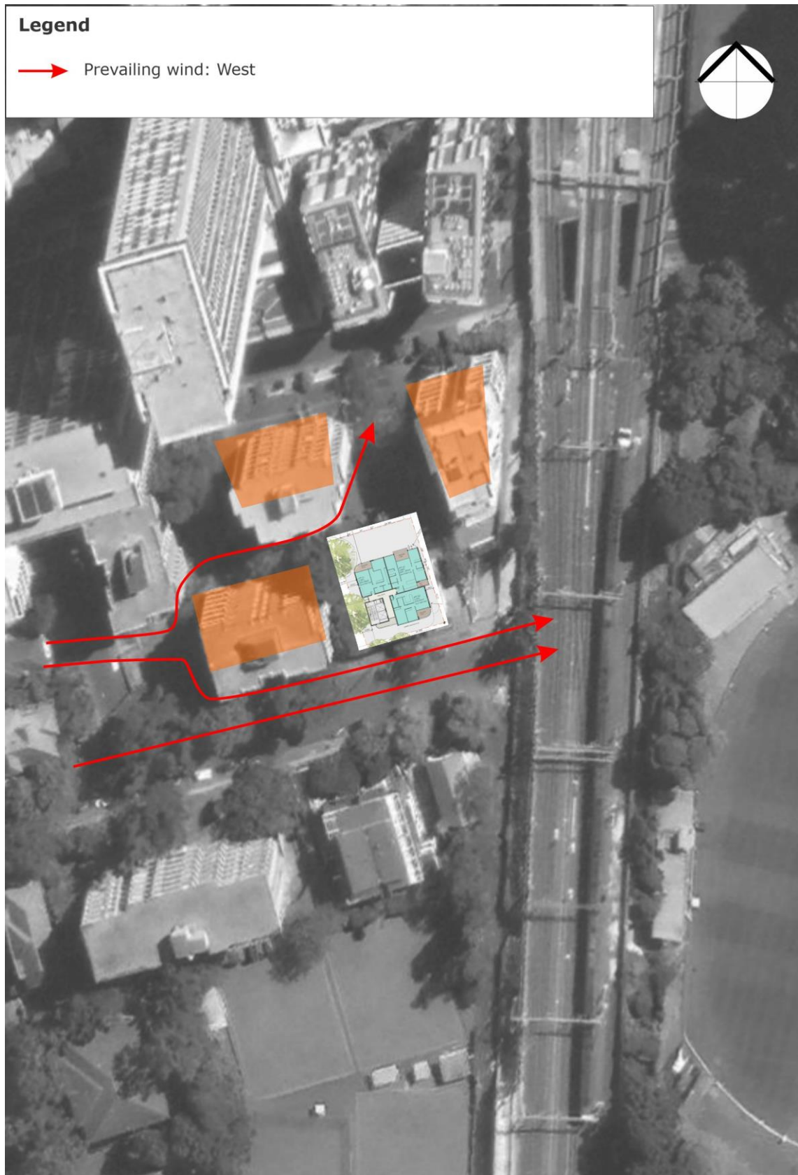
Figure 9: Flow Diagram for the Prevailing Westerly Winds
