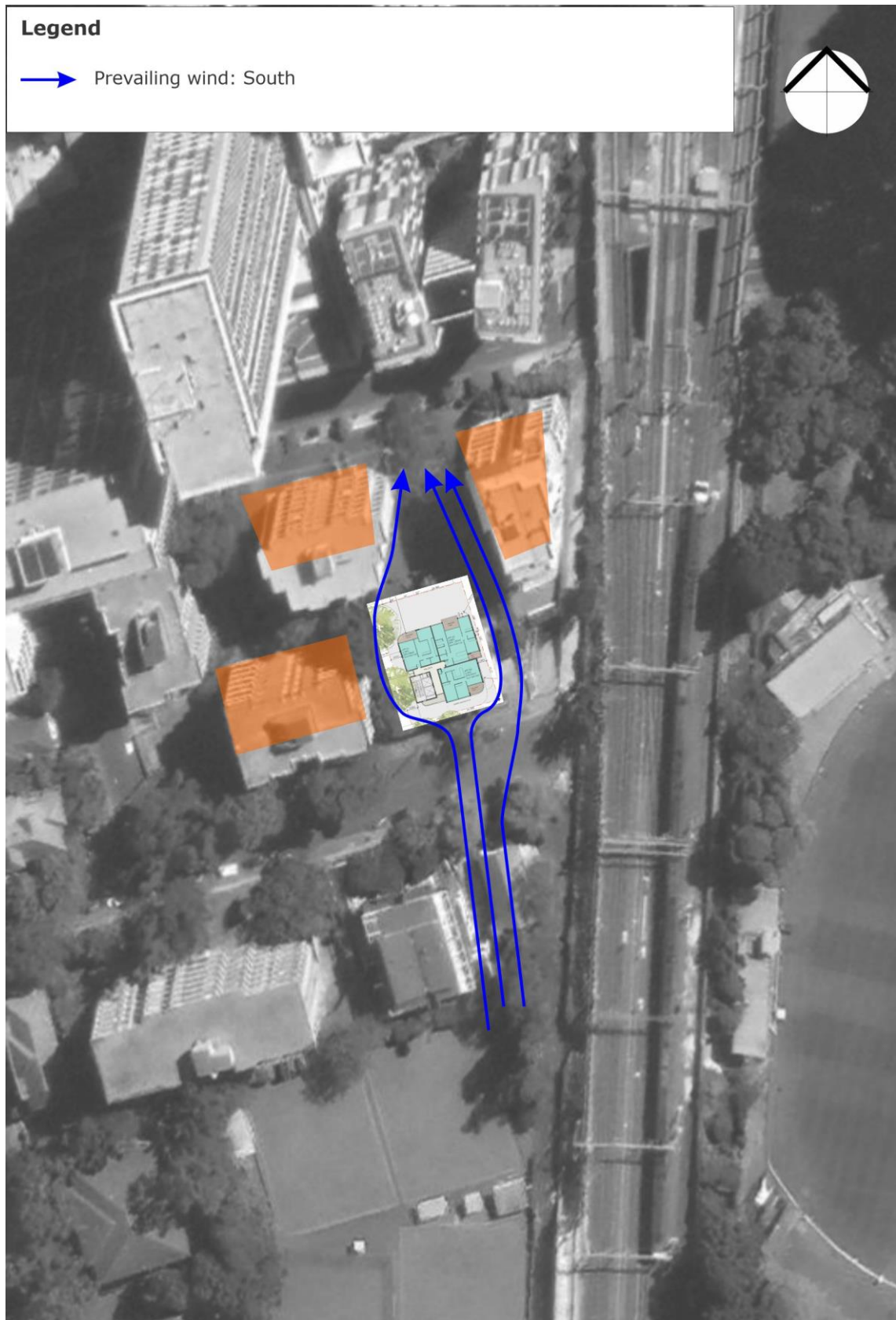
Figure 10: Flow Diagram for the Prevailing Southerly Winds
